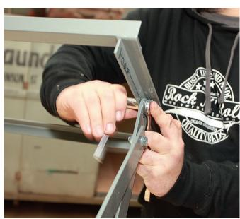
Slide the third bolt through, again not forgetting those washers between each metal surface. Ensure the lower seat rest is pointing in the right direction. Tighten the nut and bolt using the 13mm and 17mm spanner / socket
