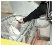
Don't forget to check that the lower support structure is also straight using a set square. Mark the position of the holes to be drilled through the wheelarches for the M10 bolts to drop through
