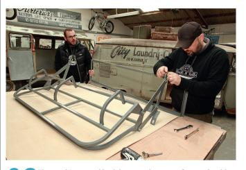
The two hinges and both lower and rear seat frames should now be united and nipped up tight. Flip the seat over so it's resting on its rear frame and extend the hinge so that sections 3 and C are exposed at the bottom
