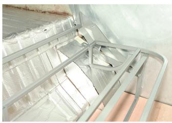
Position the seat roughly upright so the bolt-in feet are level with the wheelarches. We used a strip of masking tape to avoid damaging the sound deadening, and also so we could mark the position of the holes to be drilled for the M10 high-tensile bolts. It should sit squarely so the 'arches support it, and obviously be central in the load space
