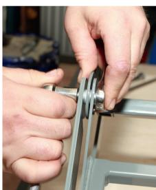
Tighten both sides using a 13mm socket and 17mm spanner
