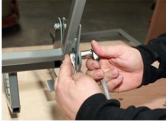
Screw on the Nyloc and then tighten with the 13mm and 17mm socket / spanner. Repeat on both sides
