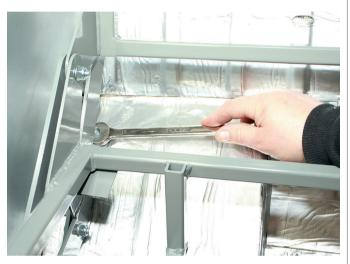
With the help of your able assistant, wrestle the bed back into position and drop the bolts through the holes. What you can't see here is that Lee is underneath the Van with the socket ready to nip up the Nyloc from below. Repeat for the other side
