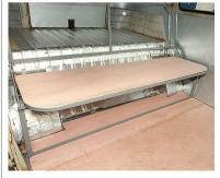
with two 9mm ply boards that form the base and back rest of your seat. Nick radiused the corners as shown freehand using a jigsaw. If you have never done this job before, we suggest you make a stiff card template, then flip it over so both corners match
