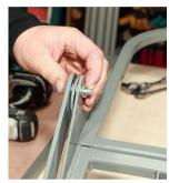
Repeat this process on the other side and unite the hinge to the rest of the framework. Pass the bolt through the back rest fixing first, add another washer, then pass the bolt through the lower seat frame fixing and add another washer. You should end up with bolt head, washer, hinge, washer, back rest, washer, lower squab, washer, nut in that order
