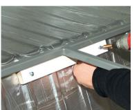
To add some extra support to the back of the bed, Nick then made a stop out of some 50mm carcassing / sawn timber. Go very carefully here with the drill as on almost all Splits and all Bays the fuel tank sits right behind here. Ensure the screws to hold this in place are suitably short
