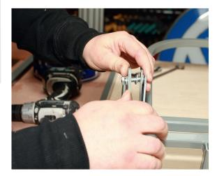
you're looking at the front of the seat, slot the first pair of the M8 bolts through the hinge with markings 1 and A. Don't forget to add the supplied washers both outside and inside the hinge as shown
