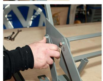
Insert the next bolt through both section 2 and B on the left and right hinges into the back rest plate. Don't forget those washers between any metal surfaces
