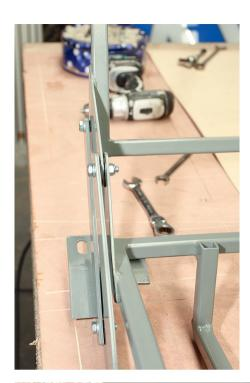
After ensuring everything is nipped up nice and tight, stand the seat up to inspect your handiwork. You can see here how the washers are a vital part of the design as they permit enough room for the hinges to slide without interference.
