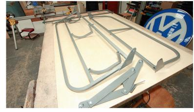
Lay the bed sections out and acquaint yourself with the left hand and right hand-specific parts. Lee kindly writes on the bed frame and hinge sections in pen – 1, 2 and 3 on the left, A, B and C on the right. Altogether you should have five separate metal pieces to make up the bed
