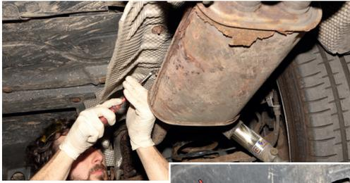
**08** Now head under the Van. You need to remove any heat shields or plastic under-body covers that prevent access to the floor. There are a variety of 10mm and 13mm bolts securing these, as well as those pesky, rusty trim clips we mentioned in the intro. Pliers and screwdrivers are your friends here
