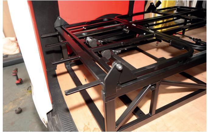
**12** Measure 260mm in from the rear step cover and position the lower back stay of the seat accordingly. Have a friend hold the seat in position and try to extend it fully into a bed, ensuring it clears both side panels freely. If you've used 6mm ply panels or backing foam, your trim could protrude further out so it's worth checking now. Our frame was positioned 50mm square from the wheelarch to clear a crossmember beneath
