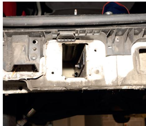
**07** Insert the captive nut plates that slide into the chassis rails. If your Van has a tow bar attachment in here, you can still use the Rusty Lee fitting kit, just without these plates
