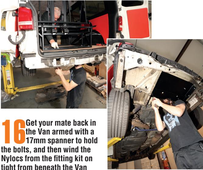
**16** Get your mate back in the Van armed with a 17mm spanner to hold the bolts, and then wind the Nylocs from the fitting kit on tight from beneath the Van
