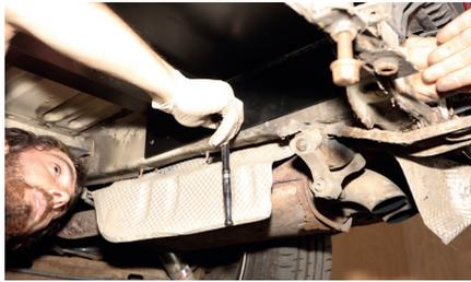
Use a dab of copper slip on the bolts and ensure they have really gripped in the captive nuts before you let go of the bracket. Do the same on the other side
