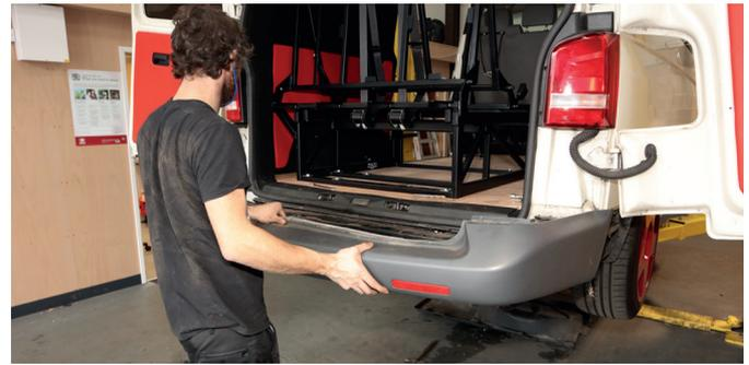
**20** Then slide your rear bumper back on, ensuring the pegs line up with the front mounts in the 'arch liners. Replace all of the Torx screws you took out earlier
