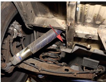
**18** The other fixing was located 130mm from the outside of the bed frame. Be sure to use washers both top and bottom on these additional fixings
