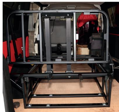
**15** Align the bed over the holes and drop all six M10 bolts through using the supplied spreader plates on top
