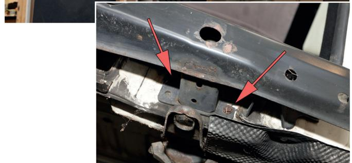
**03** Then undo the T20 / T25 Torx screws (two visible in the back 'arches' / two underneath the 'arch liners)
