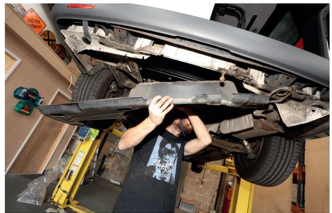
**21** Pop the plastic undertrays back into place and secure with all of the 10mm bolts and new lock washers throughout. Don't forget to replace your spare wheel and hanger as well
