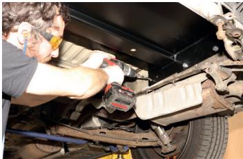
Tighten the four high tensile (8.8) stainless bolts supplied in the fitting kit each side. When you're done, you should have eight solid fixings in the chassis rails
