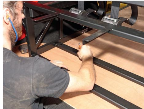
**13** Once you're happy the frame is in the right place, mark the fixing points on the floor using the pre-drilled holes in the bed frame. There are six in total
