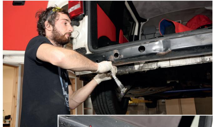
**02** You need to remove your rear bumper so start by popping off the top trim pieces inside the doors, removing the plastic screw-in trim clips with an Allen key (two up top, three beneath the Van)
